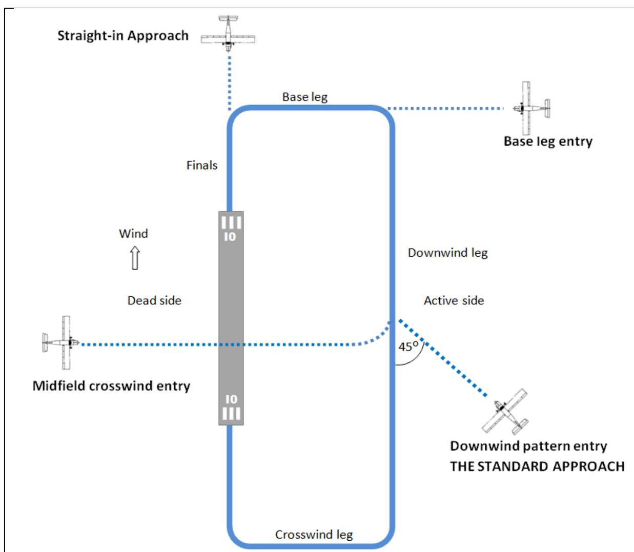
Figure 2: Circuit pattern entry possibilities
