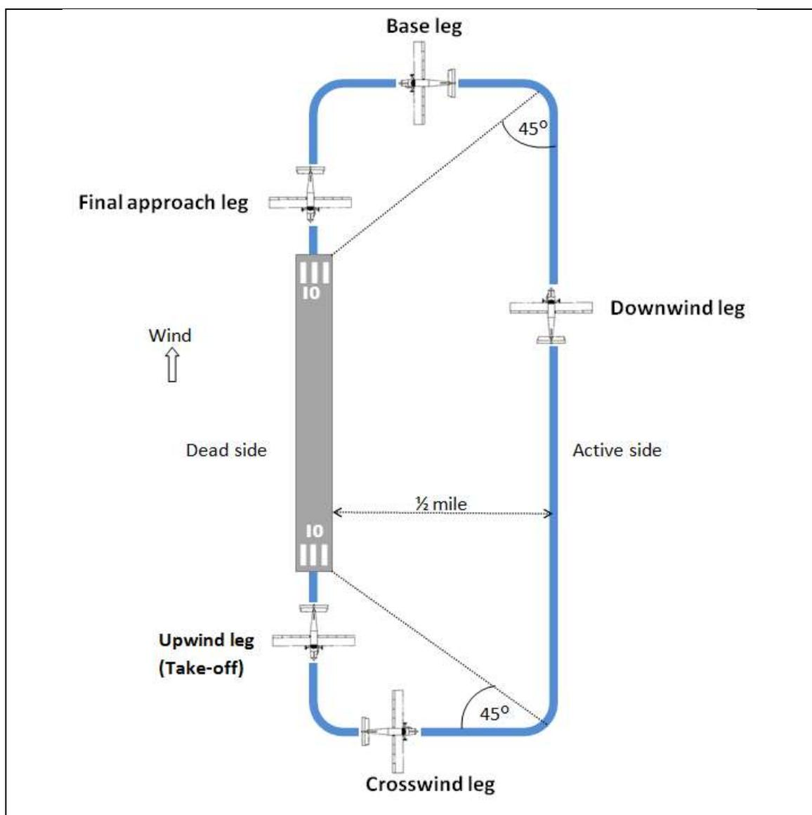
Figure 1: The standard traffic pattern for a circuit
