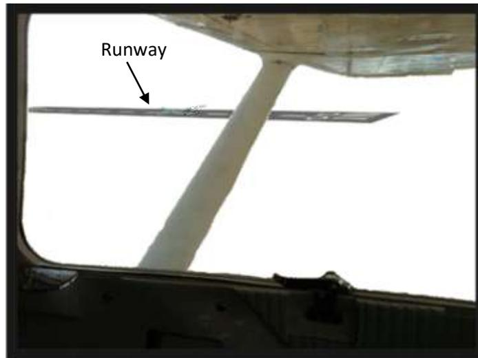
Figure 3: The correct distance from the airport
